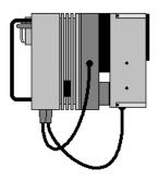
AO-8 with CFW8A Connect the AO-8 to the I2C-AUX port on the camera.
