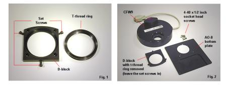
2. Use four 4-40 x 1/2 inch socket head screws to attach the AO-8 bottom plate to the CFW9 with the D-block in between as a spacer. (Fig. 2)
