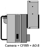
camera as a spacer to allow the AO-8 to clear the button head screws around the edge of the CFW9 (See Appendix B for details). Attach the AO-8 bottom plate to the filter wheel in this orientation with the D-block in between as a spacer, making sure that the smooth,
