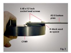
Note: It is important that you do not use screws longer than 1/2 inch as the threaded holes in the CFW9 cover plate are blind (i.e., they do not go all the way through) and 1/2 inch screws will just fit this configuration.
