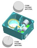
prevents the paddle from moving. The AO will try to center the paddle when first powered up so <u>it is</u> <u>important that you remove the foam before</u> <u>connecting the AO-8 to the camera or the motors</u> <u>could be damaged</u>. The first piece can be removed from aperture of the AO-8 housing by simply pulling the tissue used to line the foam insert. The second piece is inside housing and can be taken out when you remove the bottom plate in preparation for installation on the camera.
