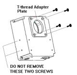
The T-thread adapter plate may be left off for shipping. If so, you can easily install it with the hex head screws and hex wrench provided. The smaller hex wrench is for removing the bottom plate from the housing. <u>The smaller wrench also fits the two hex</u> <u>head screws on the side of the housing that</u> <u>hold the motors. Do not loosen or remove</u> <u>these two screws.</u>
