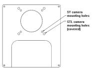
prevent light from entering the AO-8 when they are unused. <u>This tape</u> should not be removed unless you at attaching the AO-8 to an STL camera.
